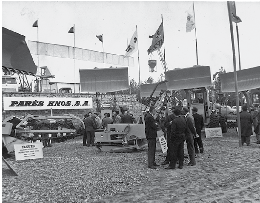
Parés Hermanos exhibition at an industrial fair in 1967. In the centre of the image stands a Davis continuous train trencher, made in the United States.
