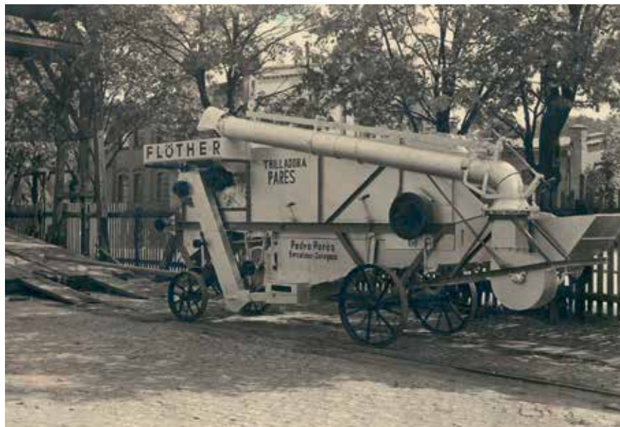
The bulky Flother cereal thresher, a notable brand manufactured in Germany, distributed by the Parés Company for several years.
