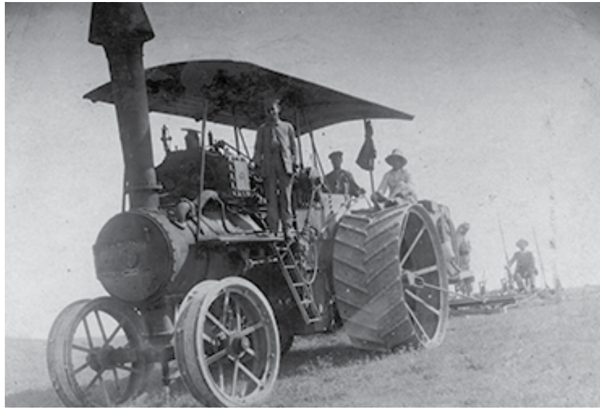
A Ruston, Proctor & Co. locomobile, a traction machine with a steam engine.
