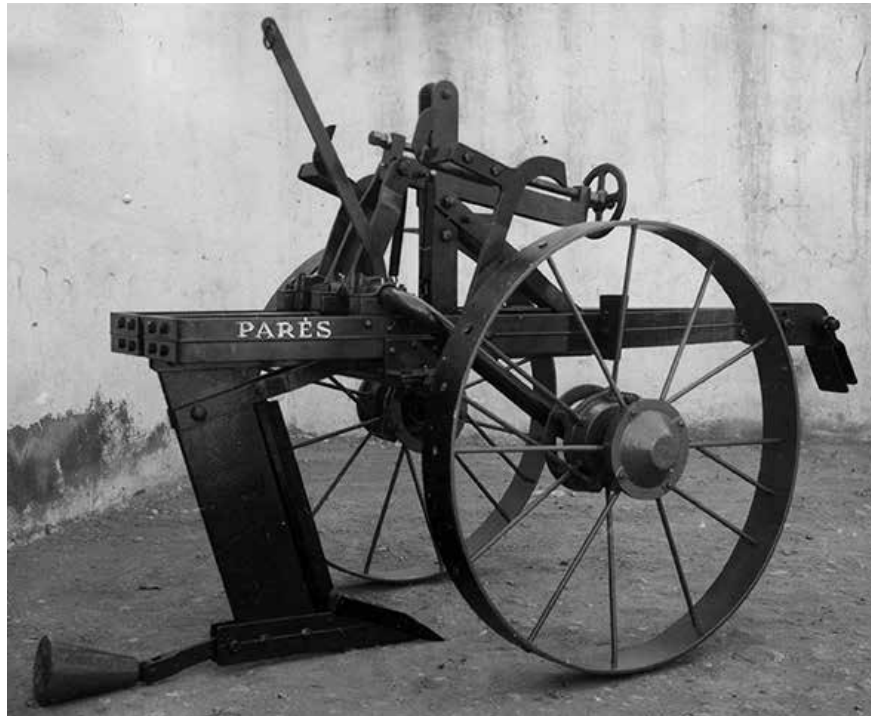
Parés chisel plough, an implement which tills the soil below the arable layer without inverting the earth. This model was made by Talleres Mariano Alegre in Huesca.
